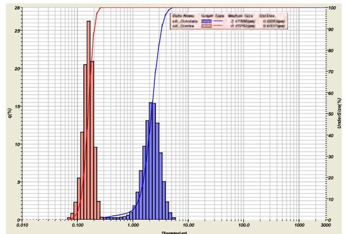
A very tight particle size distribution is produced, which results in a very stable emulsion (i.e. no creaming). When applied to emulsions with lower dispersed material volumes, it is possible to create very stable emulsions without the need for chemical stabilisation.
